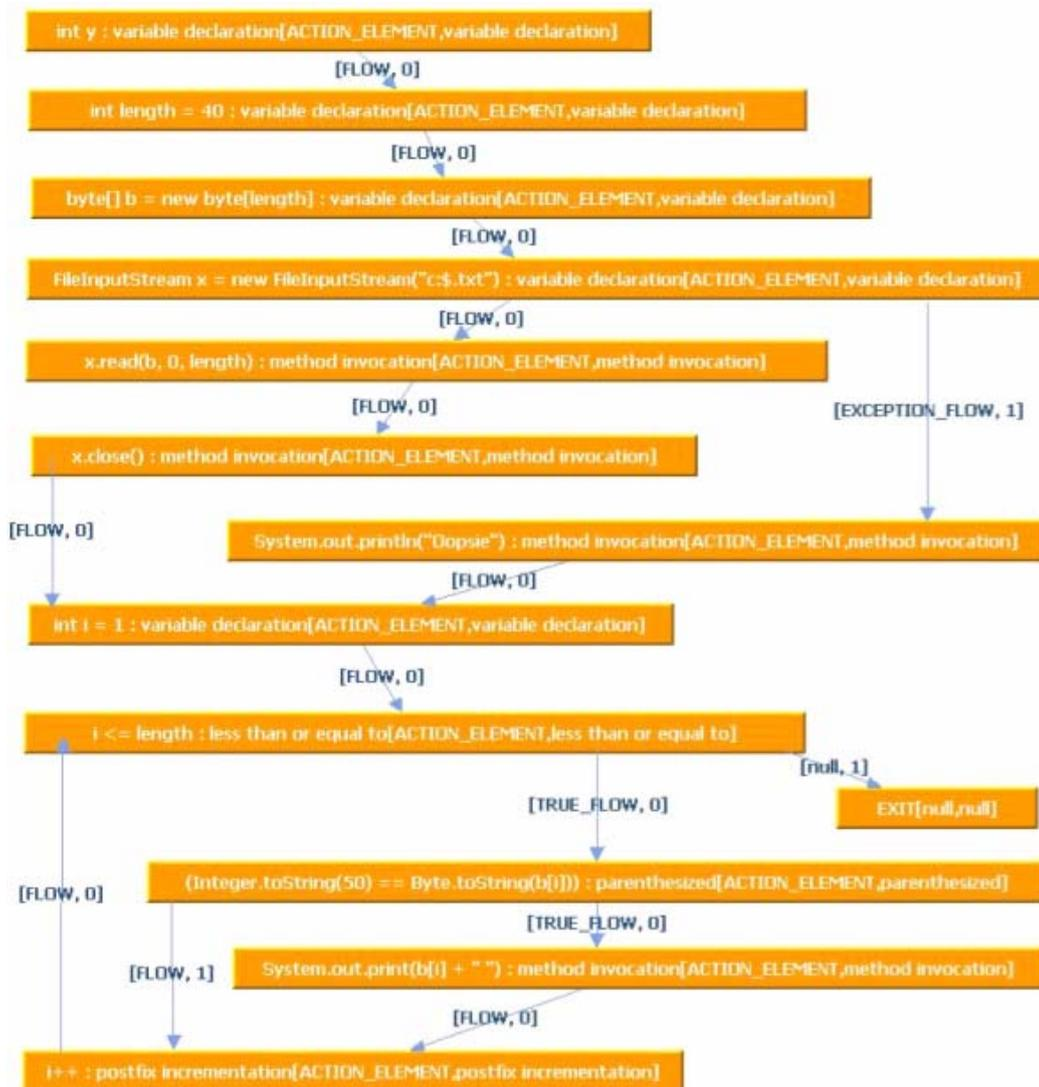
Fig. 5. CFG model of the function used in the example. Each of the nodes represents an element in the source code and the edges are jumps in the control flow (in our case, there are different types of edges – Flow, Exception Flow, True Flow, etc.)
