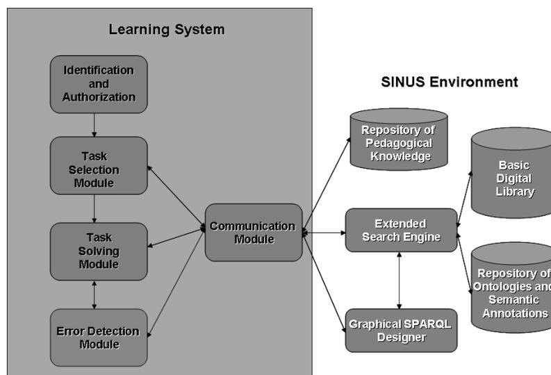
Fig. 5. The Learning System functional architecture
